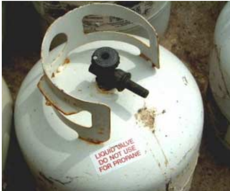
Figure 2 Modified cylinder with warning label
