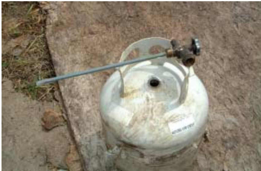
Figure 1 Modified Cylinder with dip tube
