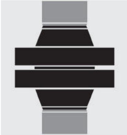
In general, flange connections consist of mating flanges, gaskets and the bolting elements. Failure to consider each and every one of these elements when doing up a flange may result in premature failure, leakage, environmental emissions and even
