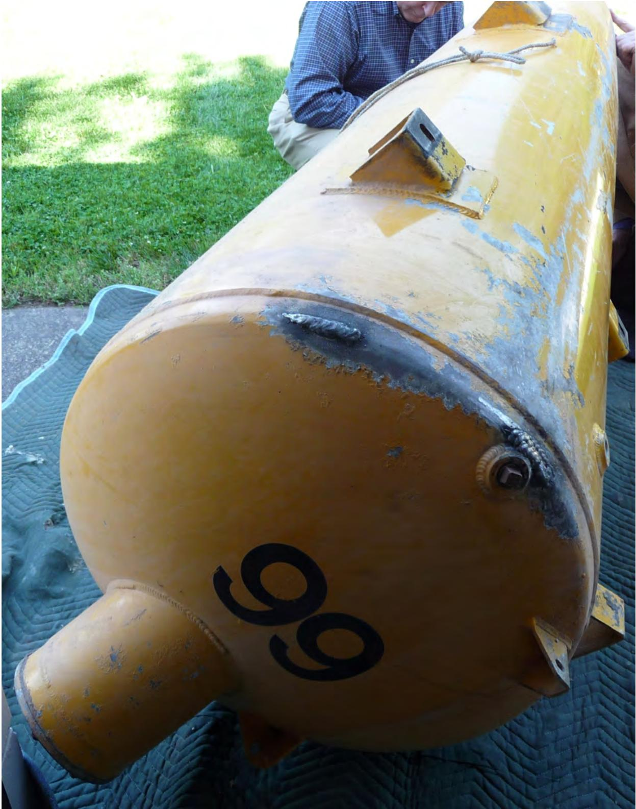
Attachment 2 - Potsko Welded Repairs
